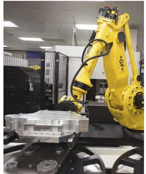
A robot loads the machines from more than one hundred open pallets.
