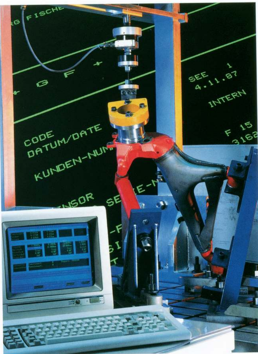
Vibration analysis of a tilted control arm for automobiles
