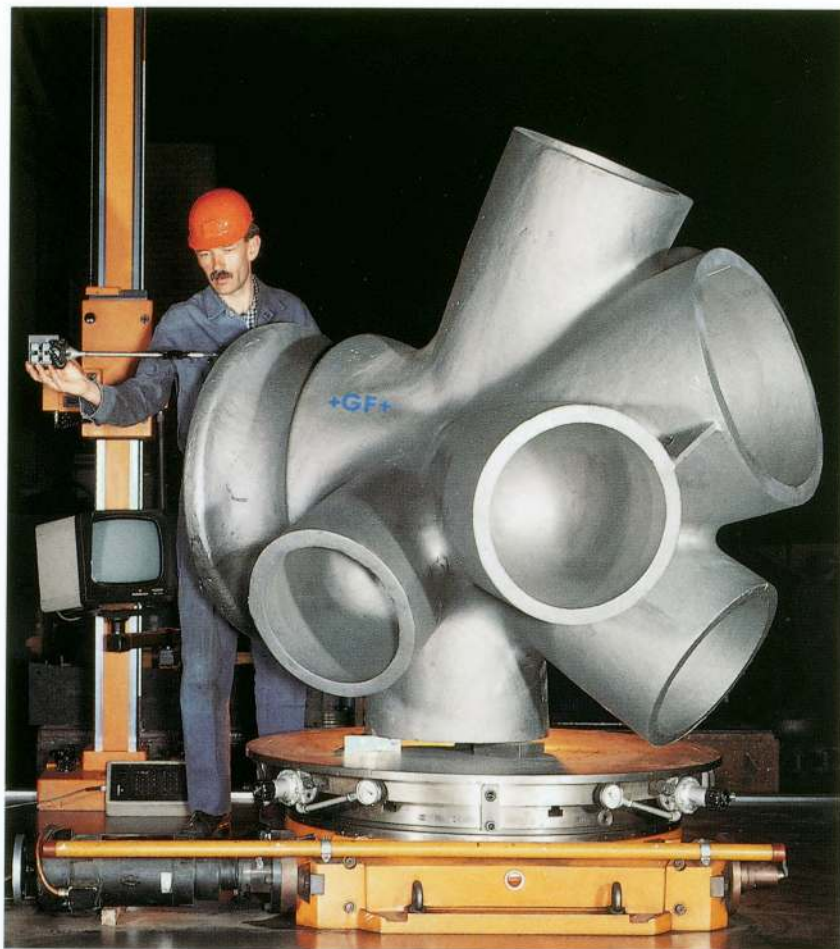
A steel cast junction for an oil rig
