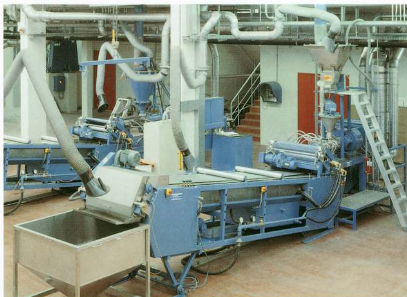
Buss Ko-kneader operated by a Swiss manufacturer of powder coatings
